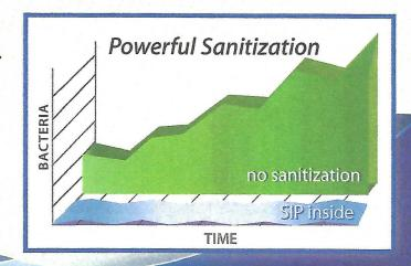
There are two technologies being used today to automatically sanitize the water cooler's reservoir on a daily basis. They are ozone made by corona discharge (as in SIP) or ultraviolet (UV) light.
